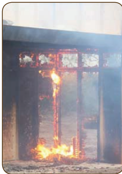
IWS-FR treated open panel with IWS-FR treated floors Reduced fire growth
