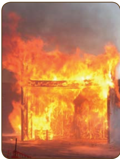
Untreated open panel with I-Joist floors Rapid fire growth
