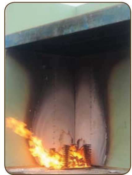
FR treated FrameProtect™ panel with FR treated floors No spread of flame and potential to self extinguish
