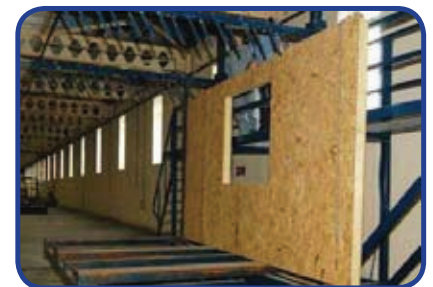
Frame UK Closed Panel Production
